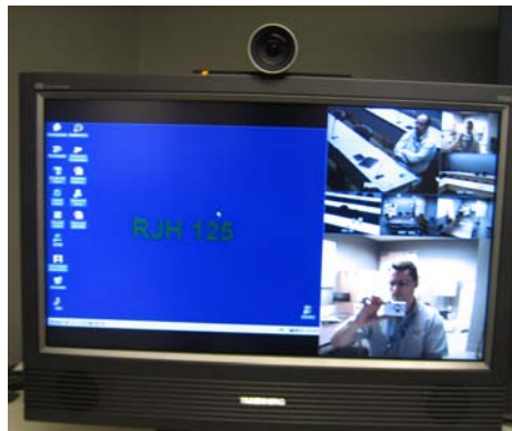
Alternative layout showing the remote PC, the connected sites (cameras) and the local camera (confidence monitor)
