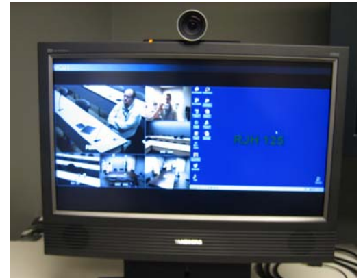
Alternative layout showing the remote PC, the connected sites (cameras) and the local camera (confidence monitor)
