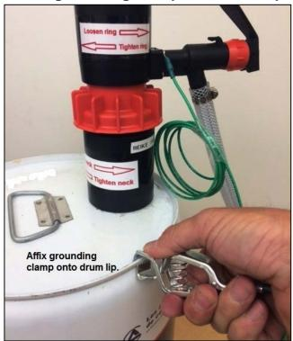
After the grounding clamp has been attached to the drum, the pump is ready for use.
