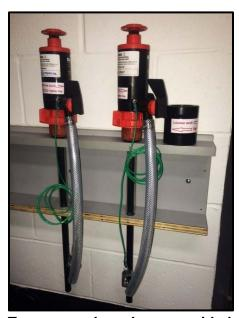
Two pumps have been provided: one for 100% (99.9%) Ethanol, one for 95% Ethanol.
