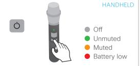
Press and hold the Mute button to turn it on/off. Press and release to Mute.
