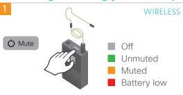
Press and hold the Mute button to turn it on/off. Press and release to Mute.
